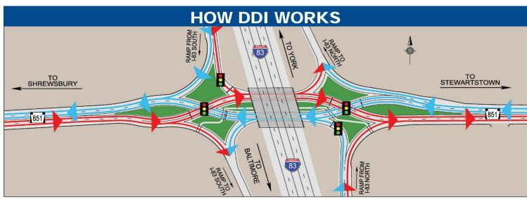
A diverging diamond interchange (DDI) is unique from a standard diamond interchange in that the side road traffic Route 851 crosses to the left side of the road at a signalized intersection prior to the bridge. This allows direct left turns from the off-ramps to Route 851 and allows for a direct left turn on to the on-ramps to I-83. The side road (Route 851) traffic crosses back to the right side of the road at a signal beyond the bridge.
