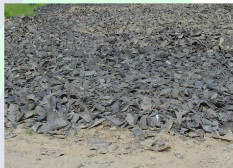
Stockpile of Tire Derived Aggregate
