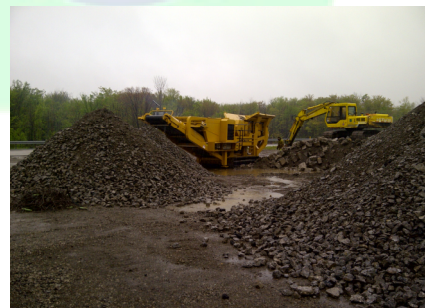
Example of concrete crushing and processing operations
