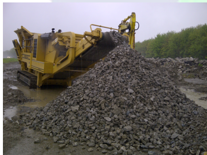
Example of concrete crushing and processing operations
