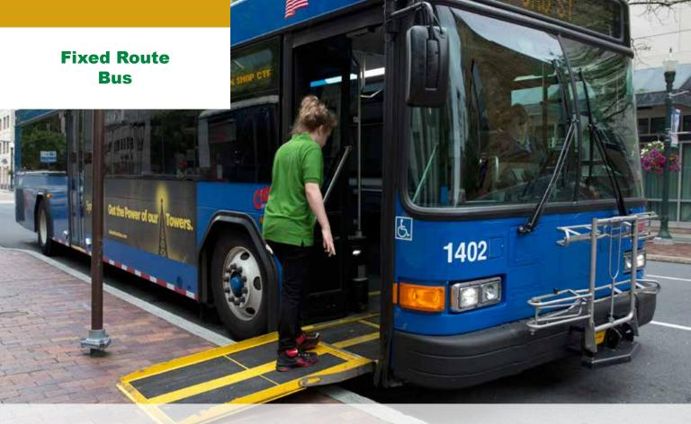
▲ Low-floor buses eliminate the obstacle of stairs. A ramp can be extended to the sidewalk.
