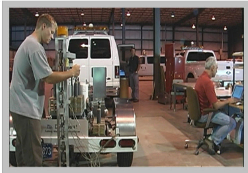
Technicians Performing an FWD Calibration at PennDOT's FWD Calibration Center
