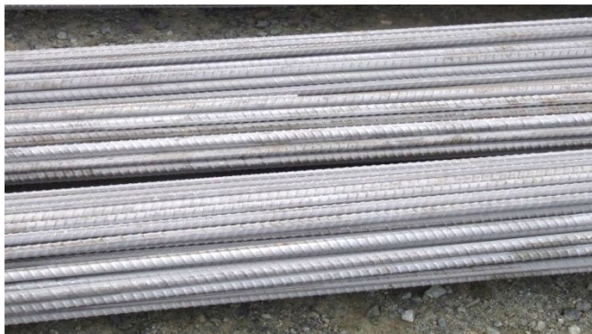
Stainless steel reinforcement
