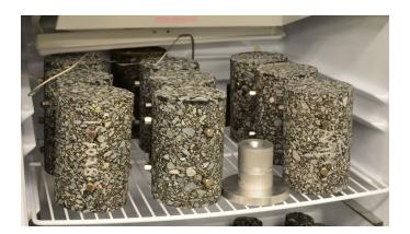
Evaluation of a mix to determine its ability to resist rutting, cracking, and deterioration *for an expected period of time*
