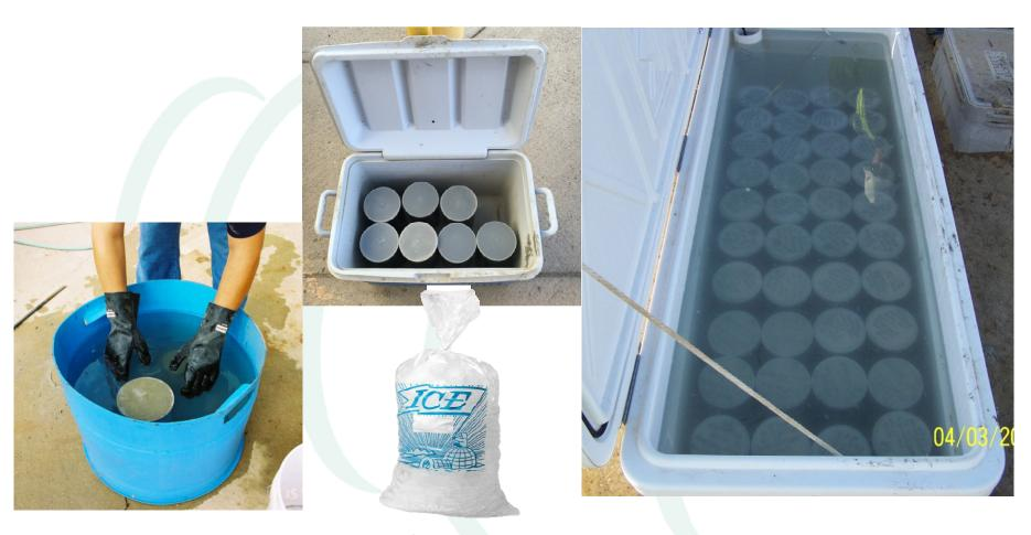
Add water (use ice if needed) and insert hi-low thermometer
