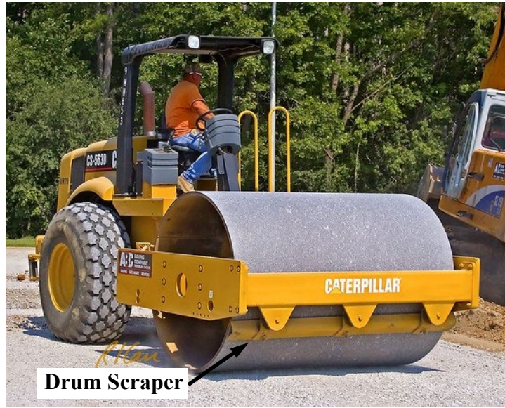
Figure 7.5-3 – Scraper on Smooth Drum Roller
