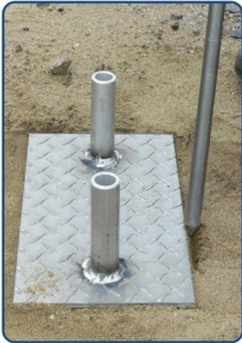
Figure 7.4-5 – Scoring Around Scraper Plate for Proper Alignment of Source Rod with Hole
