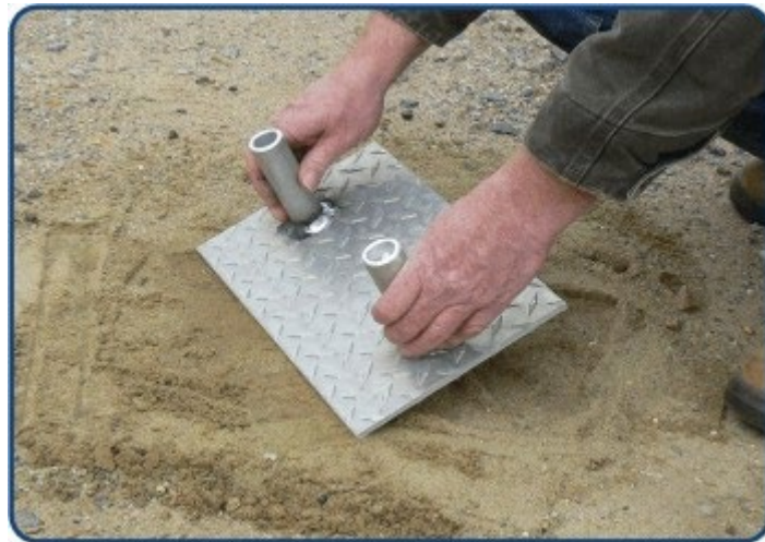
Figure 7.4-4 – Preparation of Surface with Leveling/Scrapper Plate
