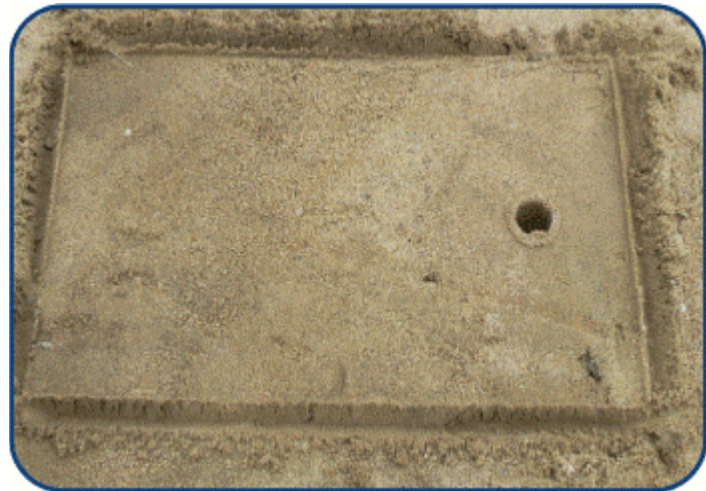
Figure 7.4-5 – Scoring Around Scraper Plate for Proper Alignment of Source Rod with Hole
