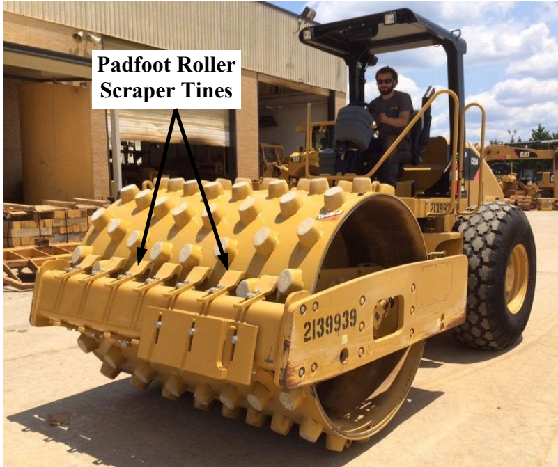
Figure 7.5-4 – Padfoot Roller Scraper Tines (Between Pads)
