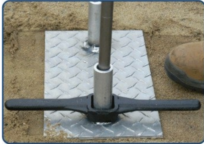
Figure 7.4-6 – Drive Rod in Plate Guide Hole with Extractor Tool
