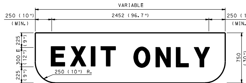
EXIT ONLY PANEL
