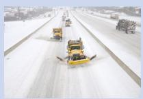
operator to get out of the truck to clean it. The **Lighted Plow Whips** innovation is designed to increase operator and motorist awareness during snowstorms and nighttime operations, by increasing visibility of the plow during whiteout conditions. The TAG is currently working with a vendor to update the lighting colors of the plow whips to optimize the effectiveness of the innovation.
