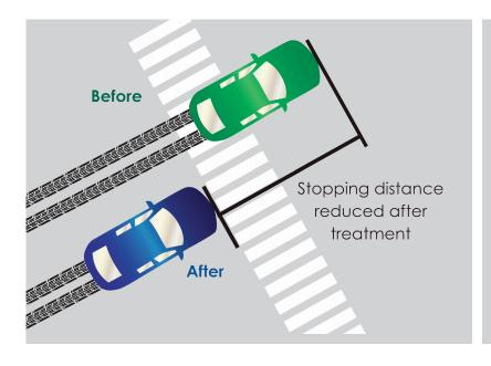
High Friction Surface Treatment (HFST) increases roadway friction allowing vehicles to stop easier and maintain control. This safety innovation dramatically increases roadway skid resistance to prevent crashes.
