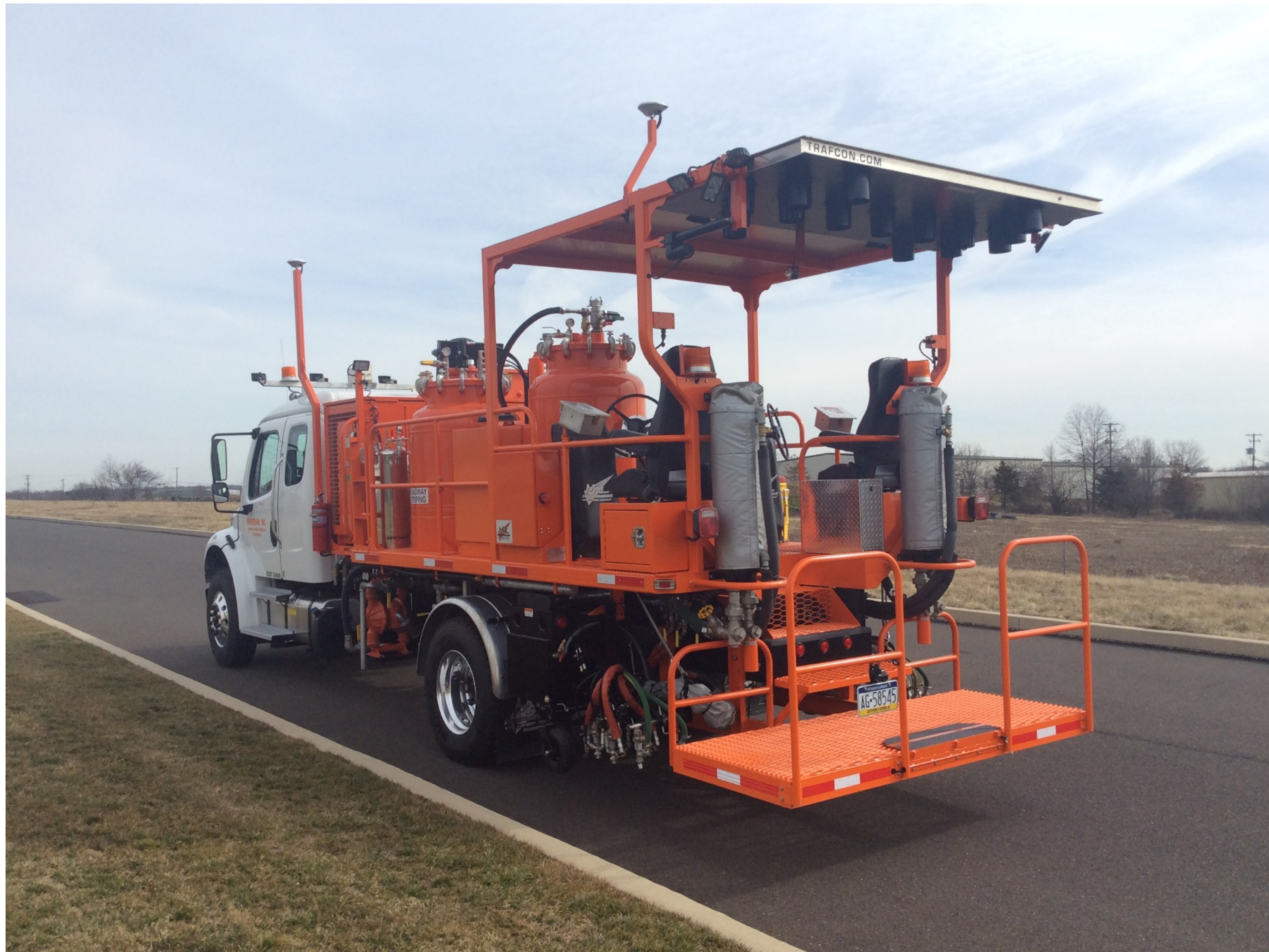
A paint truck equipped with robotic layout system.
