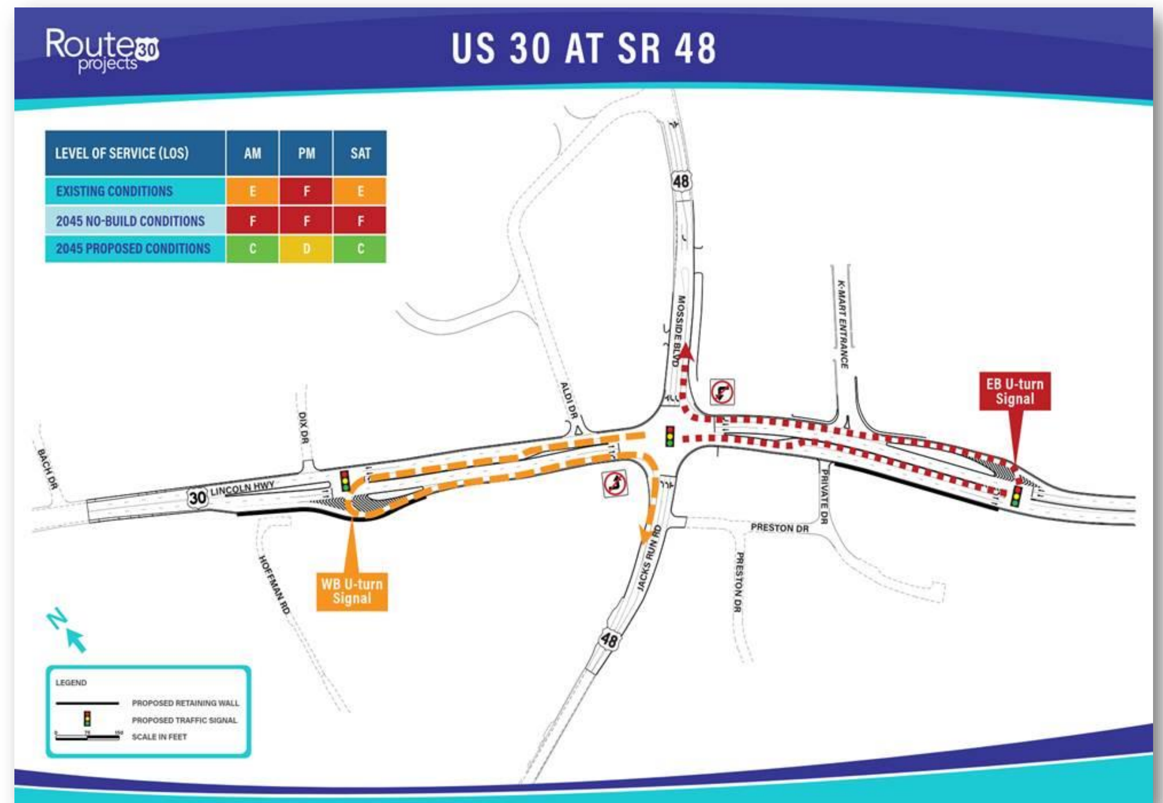
Proposed MUT Intersection concept at US-30 and SR-48, Allegheny County, PA Source: US-30 Projects, Western Section Design
