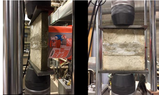
Concrete plate under cyclic loading - Source: University of Pittsburgh
