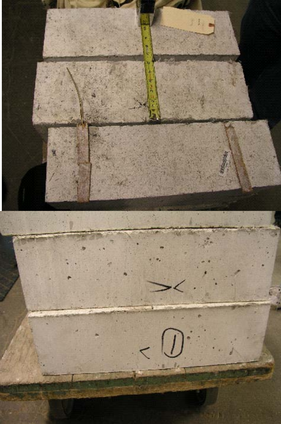
Photographs 33 and 34, The Tuf-Strand fibers in the concrete kept the beams in one piece after testing. The control beam split into two pieces.
