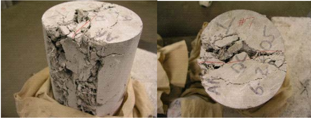
Photographs 29 and 30, The Tuf-Strand fibers in the concrete kept the cylinders in one piece after the destructive testing.
