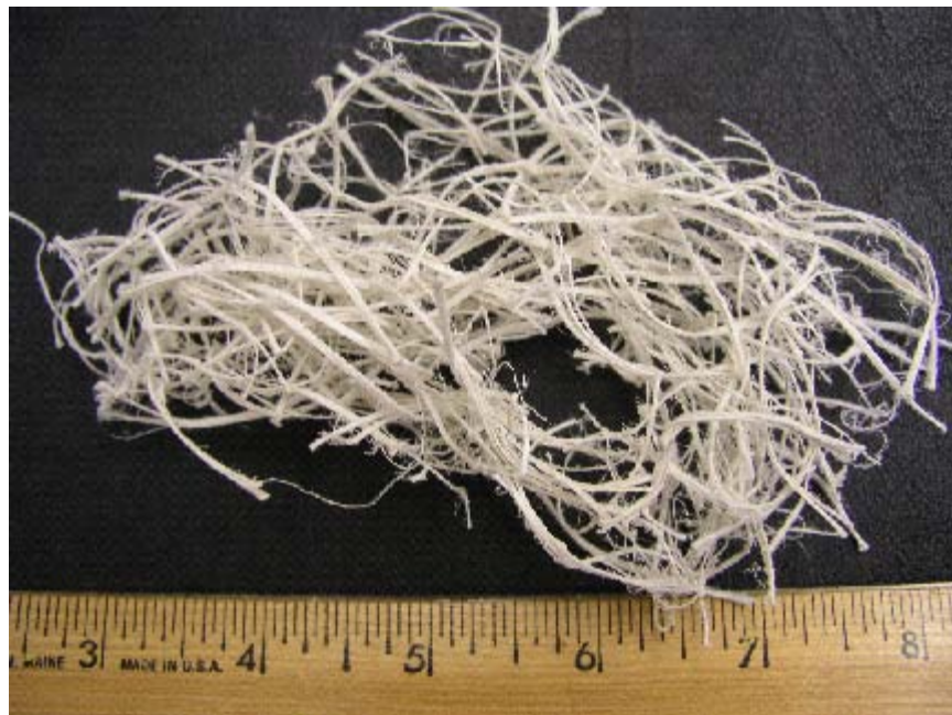
Photograph 4, These are the Tuf-Strand Fibers after they were added to a batched concrete mixture. A small sample of the fresh batched Class AA Concrete with the Tuf-Strand fibers was washed and these fibers were collected from the remaining aggregate. Note that the Tuf-Strand fibers swell and become frayed to enhance blending into the cement paste of the concrete.
