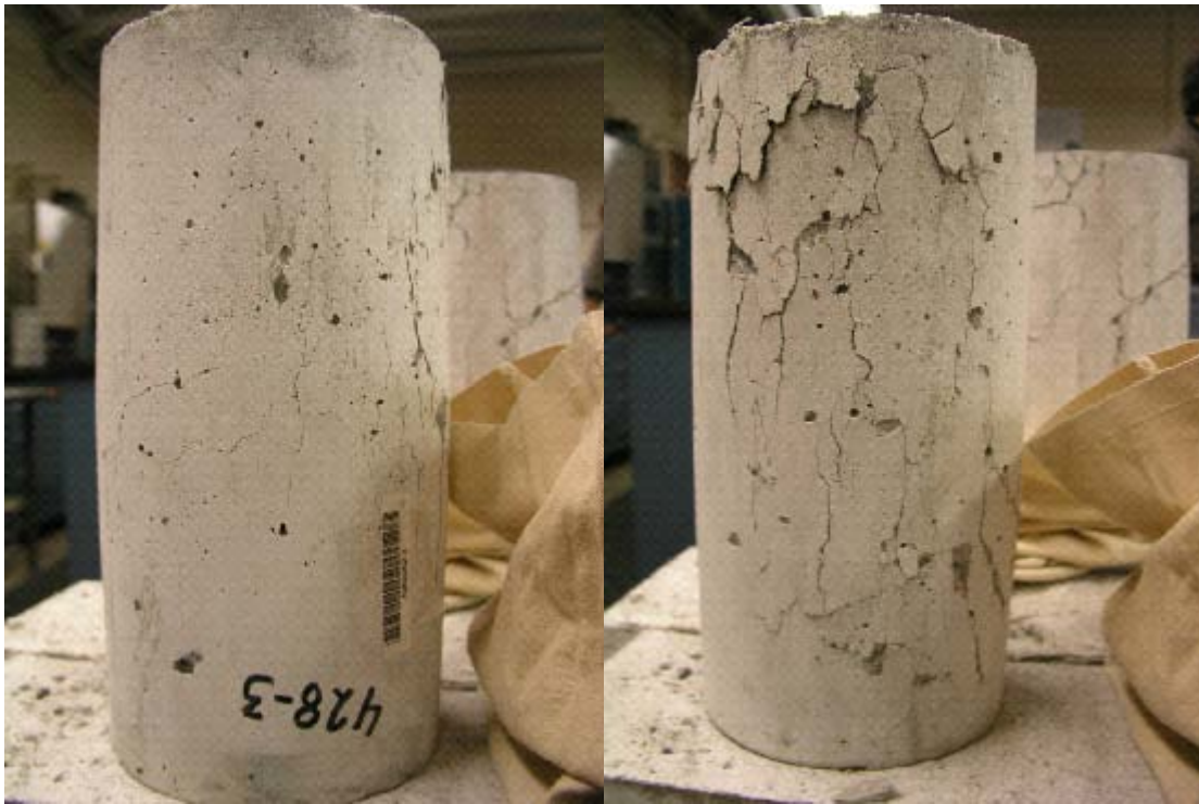
Photographs 27 and 28, The concrete cylinders fractured during testing but still maintained their shape because of the Tuf-Strand fiber additive.
