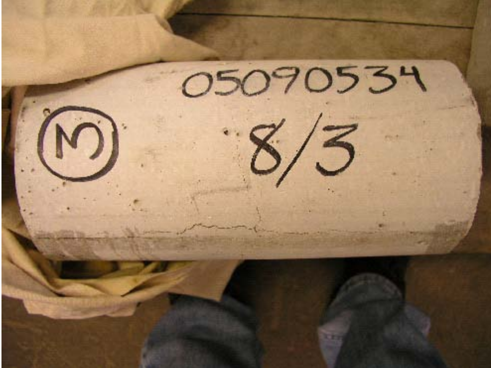
Photograph 38, This control cylinder for Class AA nearly split into two pieces.
