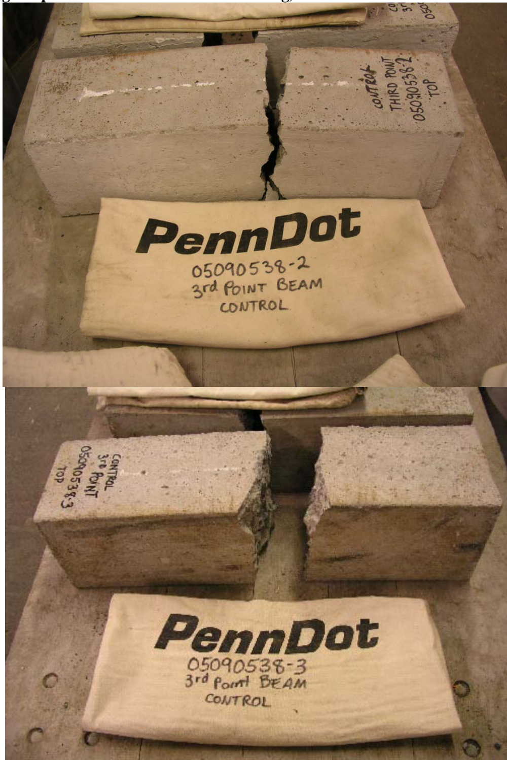
Photographs 41 and 42, Flexural test beam specimens.
