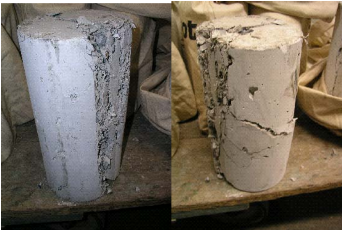
Photographs 31 and 32, The Tuf-Strand fibers in the concrete kept the cylinders in one piece after the destructive testing. The control concrete cylinder split in half.
