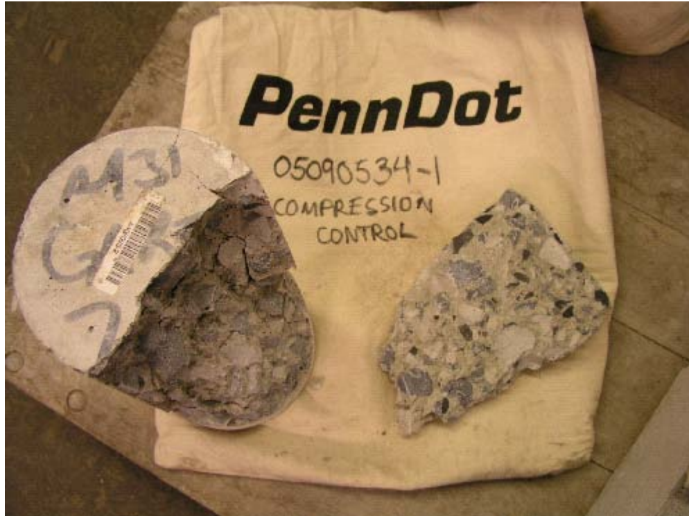
Photograph 35, This control cylinder for Class AA split into two pieces.
