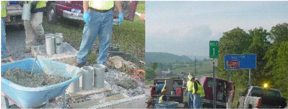
Photographs 9 and 10, Samples of the Class AA Concrete were collected in the field. Concrete cylinders were cast for both compressive and tensile strength tests. Beams were also cast for flexural testing at 28 days. Mile Marker and Informational Signs were used as land marks to locate the two concrete patches for evaluation after the construction project is completed.
