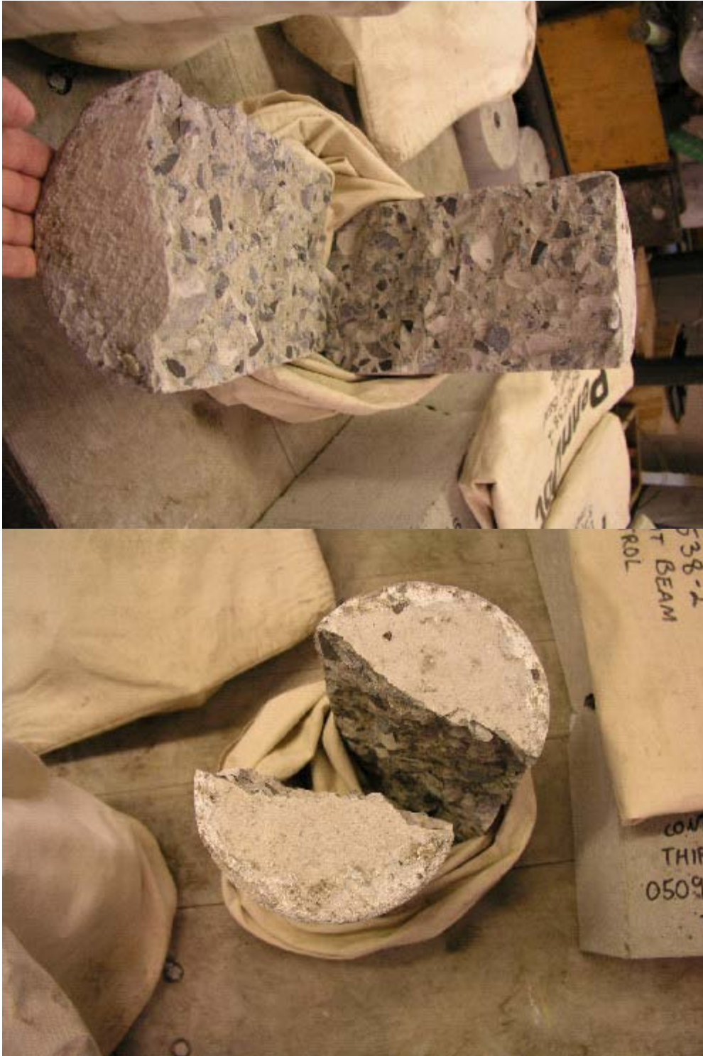
Photographs 36 and 37, The fractured control cylinder for Class AA split into two pieces.
