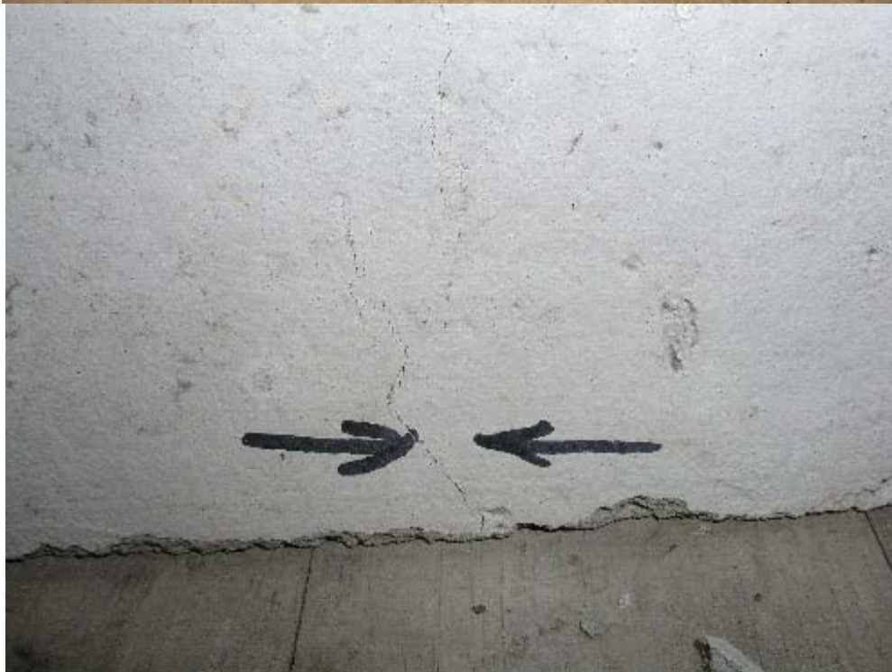
Photographs 39 and 40, The flexural test beam specimens and the line of fracture.
