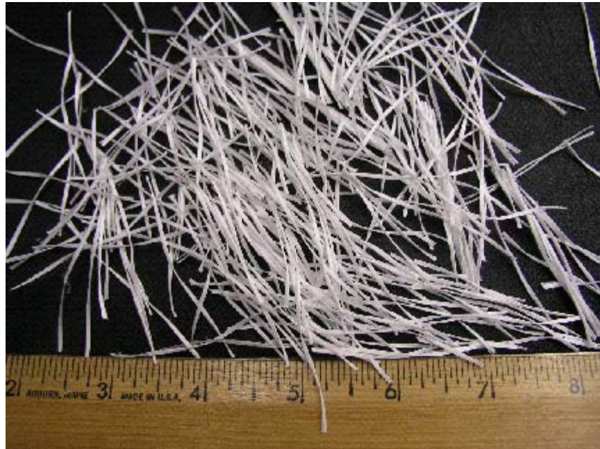
Photograph 3, These are the Tuf-Strand Fibers before they are added to the batched concrete mixture.
