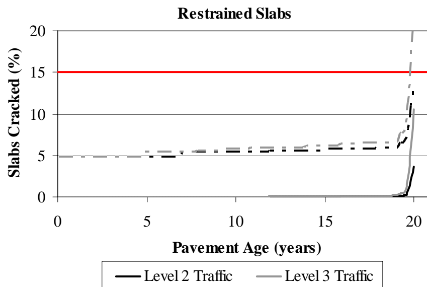
Figure 4.45. Percent cracking in the restrained slabs for Level 2 and Level 3 traffic inputs.
