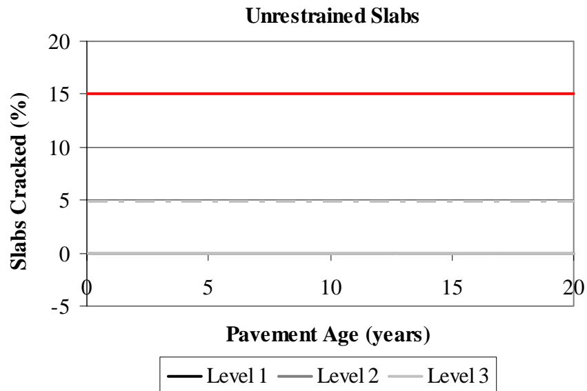
Figure 4.42. Predicted percent cracking in the unrestrained slabs.
