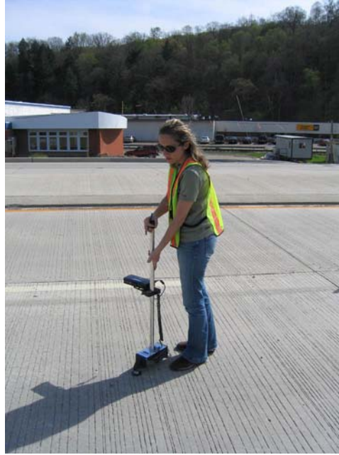
Figure 5.30. Surface profile measurements using the dipstick.
