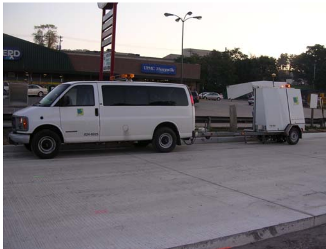
Figure 6.3. Falling weight deflectometer used on S.R. 22.
