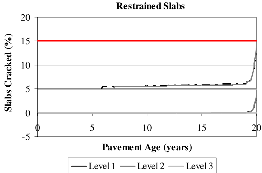
Figure 4.40. Predicted percent cracking in the restrained slabs.
