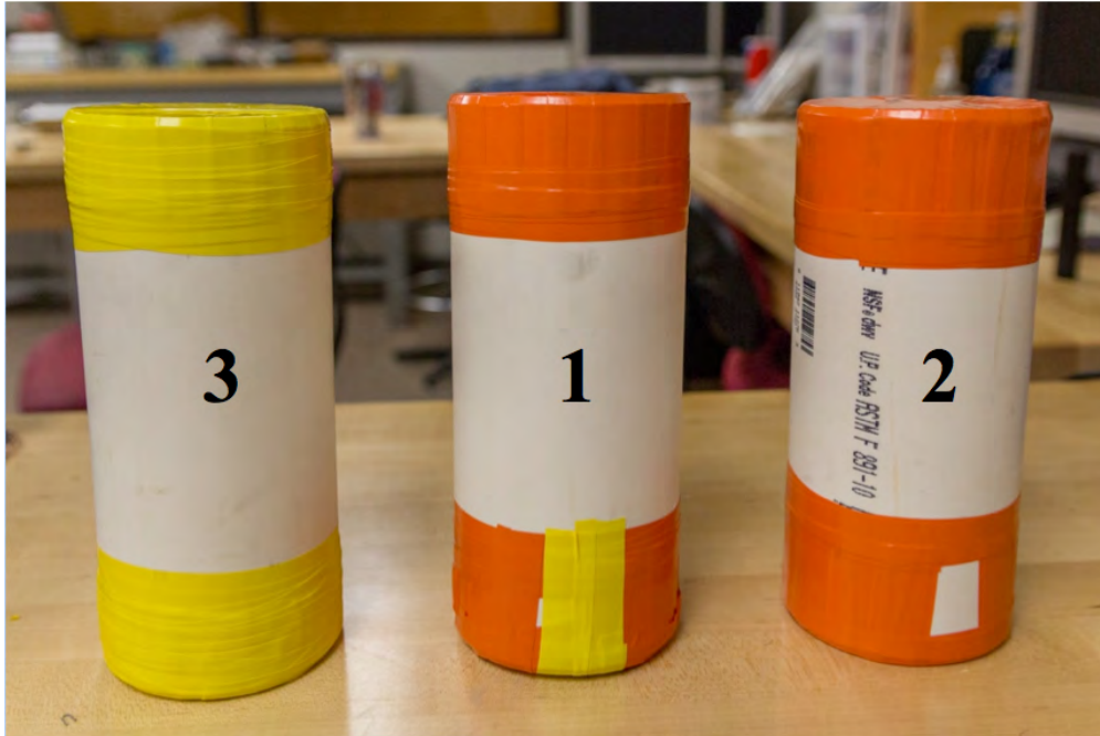
Figure 25: River Test 2 Float-out Devices Sealed for Deployment
