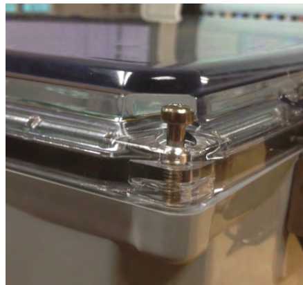
Figure 5: Captive Screws to Ensure the Neoprene Seal is Watertight
