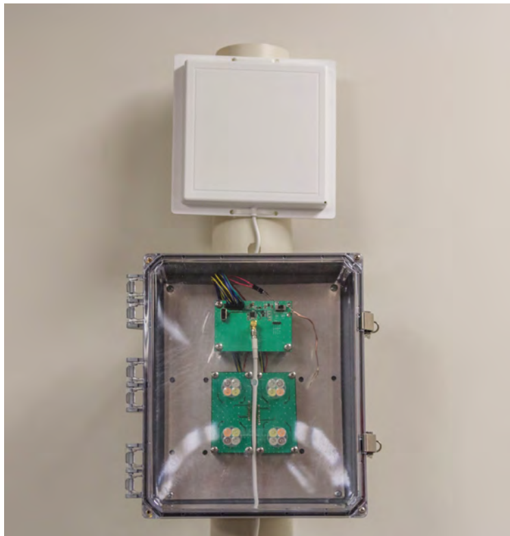
Figure 4: Receiver Enclosure with Receiver Unit, Two Light Indicators and Patch Antenna
