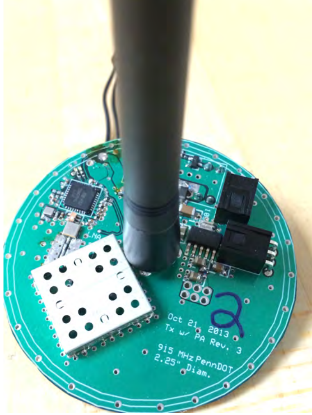
Figure 7: Float-out Device Populated Printed Circuit Board
