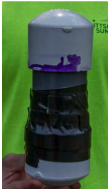
Figure 24: PVC Capsule used during River Test 1
