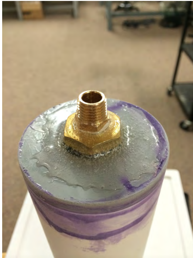
Figure 22: Float-out Device with 0.25" Bulkhead Sealed to custom PVC Cap
