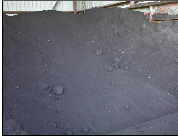
Photo 1, The pulverized shingles were stockpiled at the H&K, Bechelsville Plant under roof. The material resembled coarse black sand.
