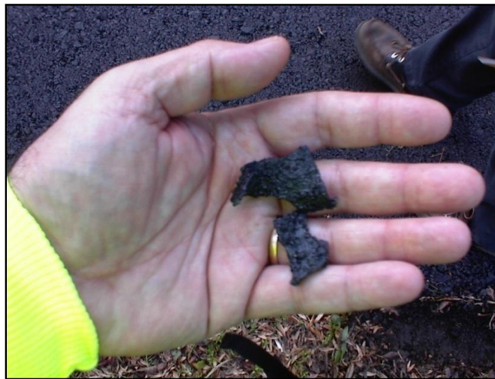
Photo 6, Pieces of shredded roofing membrane contaminant is removed during the paving operation.
