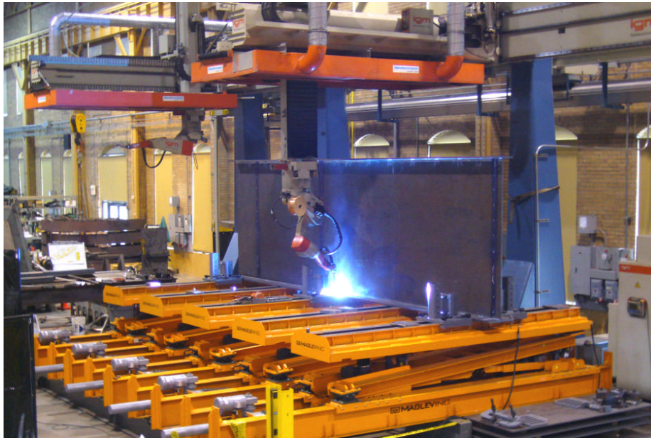
Figure 21.0 Bottom flange of 23-ft beam being welded without upper hold-downs.
