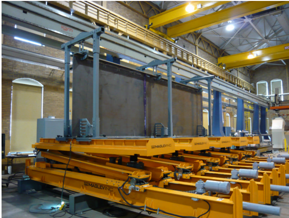
Figure 19.0 Full cross-section 23-ft beam in place with hold down fixtures.
