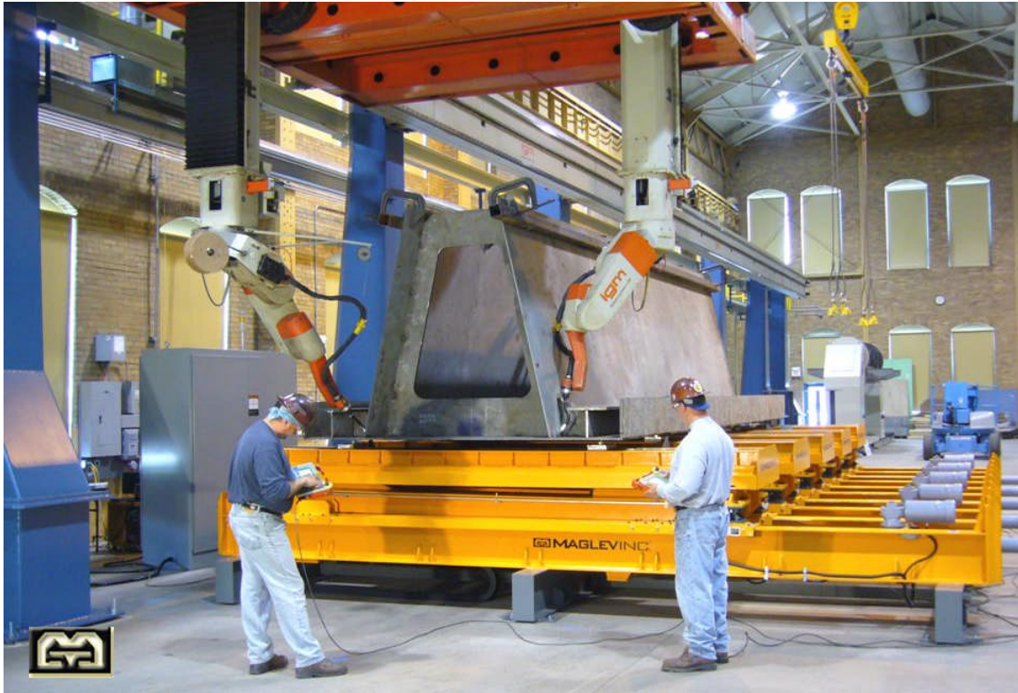
Figure 1.0 Automated fit-up table and gantry robot weld system at MAGLEV, Inc.
