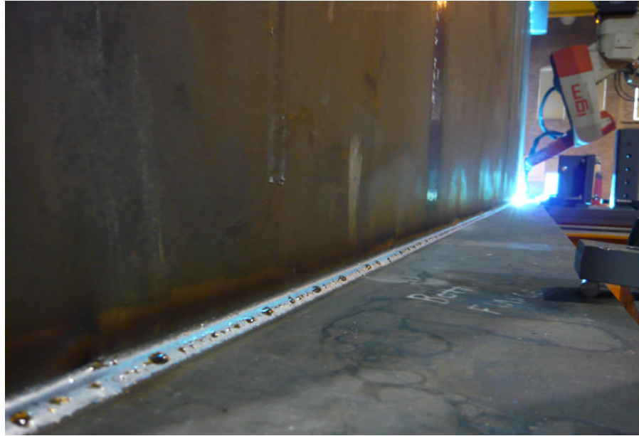
Figure 22.0 GMAW 2F welding of the bottom flange on a 23-ft beam. Some silica bubble beads are present on the weld bead surface.
