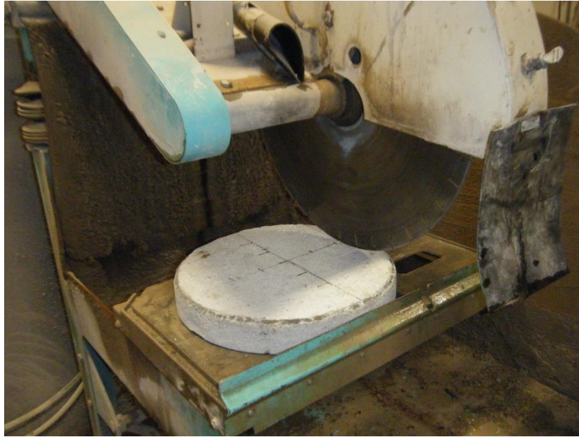
Figure 30. Mortar cubes being cut from the curing specimens.
