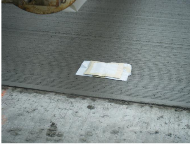
Figure 16. Field specimen for measuring the application rate of the curing compound.
