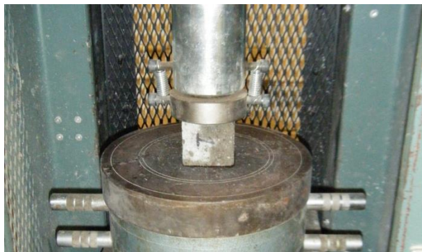
Figure 31. Typical 2 in mortar cube tested for compression strength.
