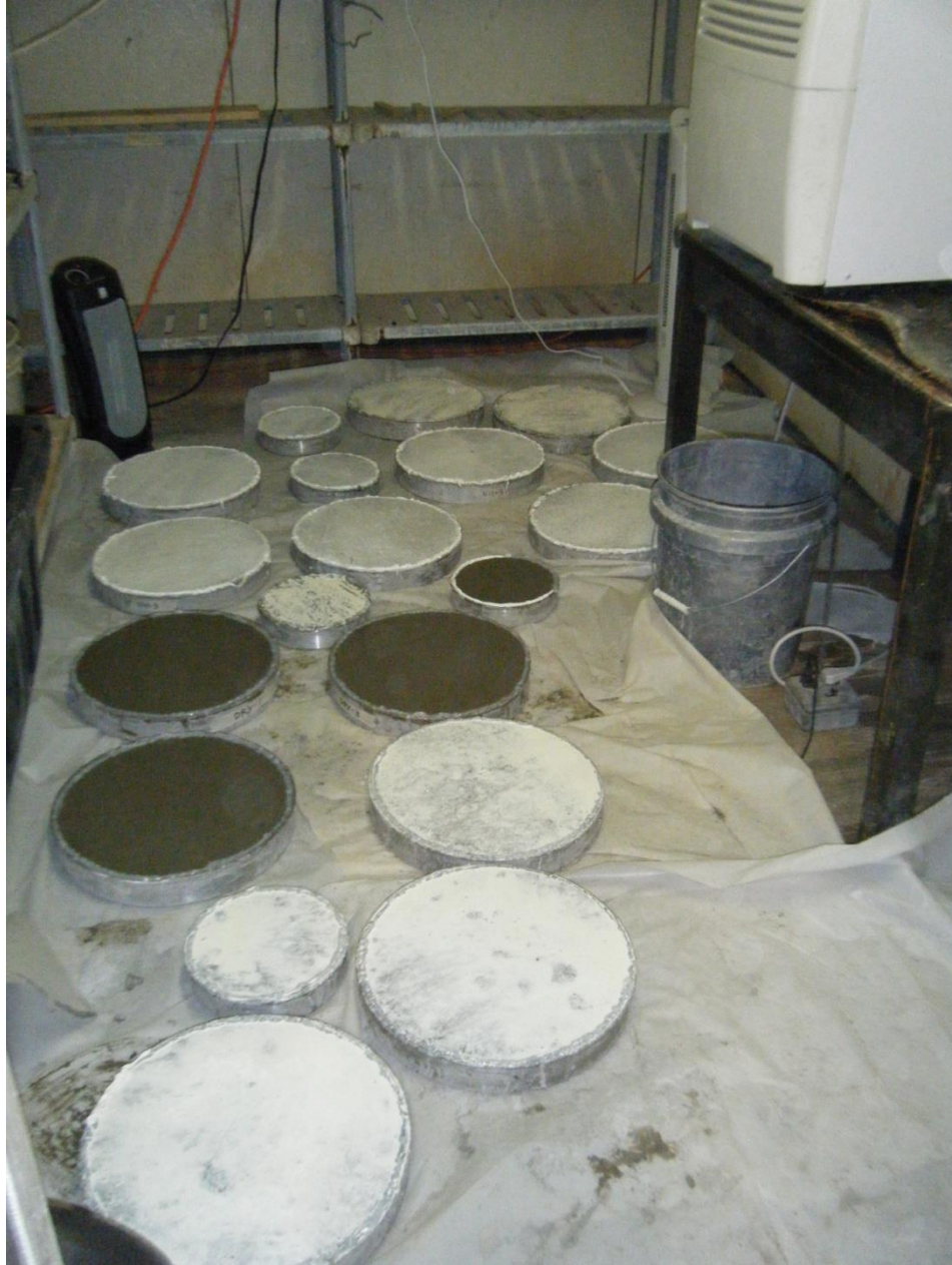
Figure 29. Finished specimens placed in environmental chamber.
