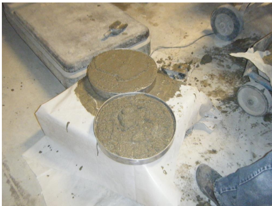
Figure 26. Mortar specimens placed in lifts on vibration table.
