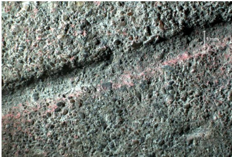
Figure 24. Wear/erosion of the pavement surface on the surface of core from US 22 in Westmoreland County, PA.
