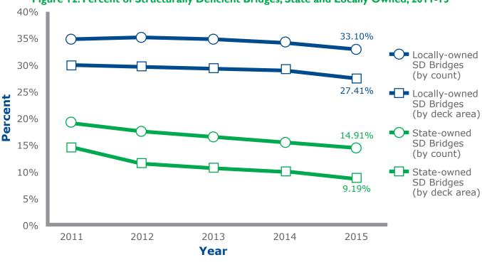
Figure 12: Percent of Structurally Deficient Bridges, State and Locally Owned, 2011-15
