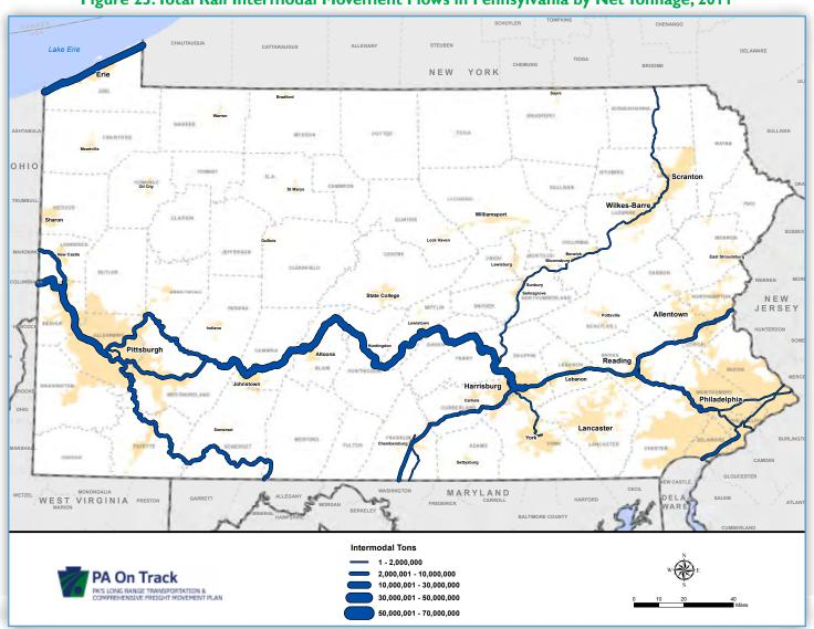
Figure 23:Total Rail Intermodal Movement Flows in Pennsylvania by Net Tonnage, 2011
