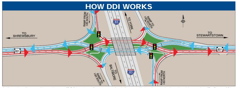
A diverging diamond interchange (DDI) is unique from a standard diamond interchange in that the side road traffic Route 851 crosses to the left side of the road at a signalized intersection prior to the bridge. This allows direct left turns from the off-ramps to Route 851 and allows for a direct left turn on to the on-ramps to I-83. The side road (Route 851) traffic crosses back to the right side of the road at a signal beyond the bridge.
