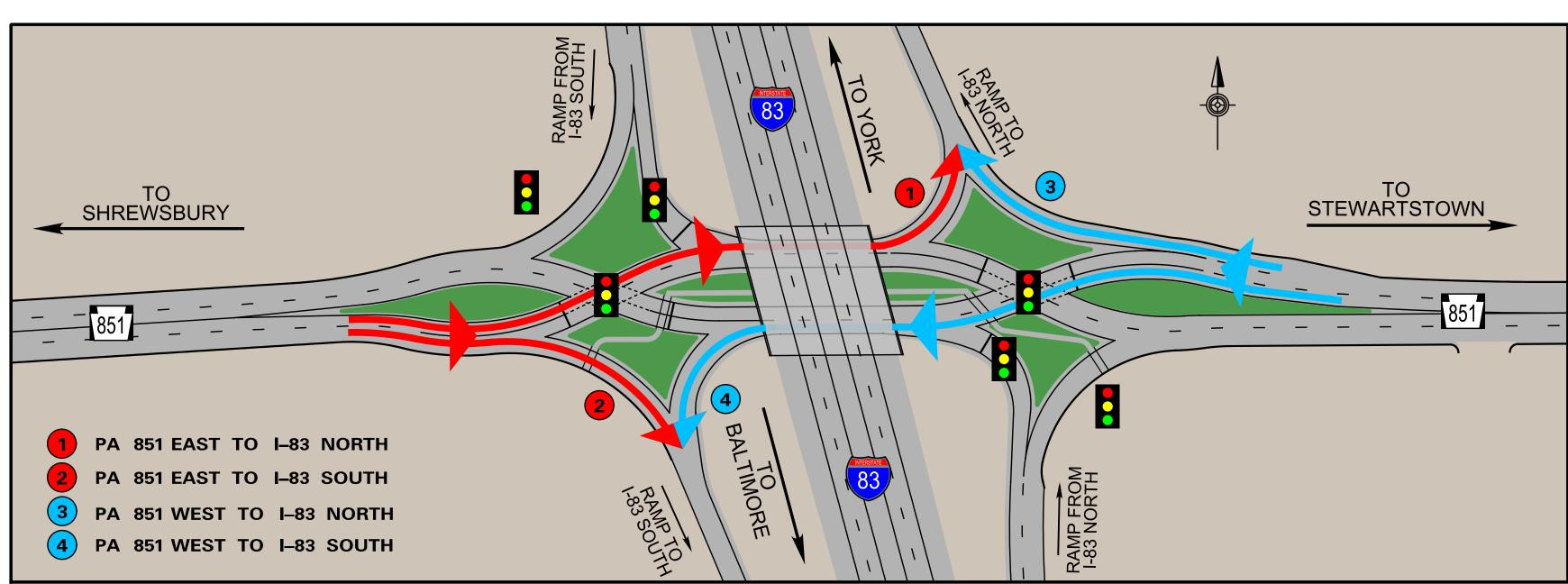
Traffic from PA 851 can turn right prior to the first signal to enter the on-ramp (movements 2 & 3) or turn left immediately following the bridge (movements 1 & 4).
