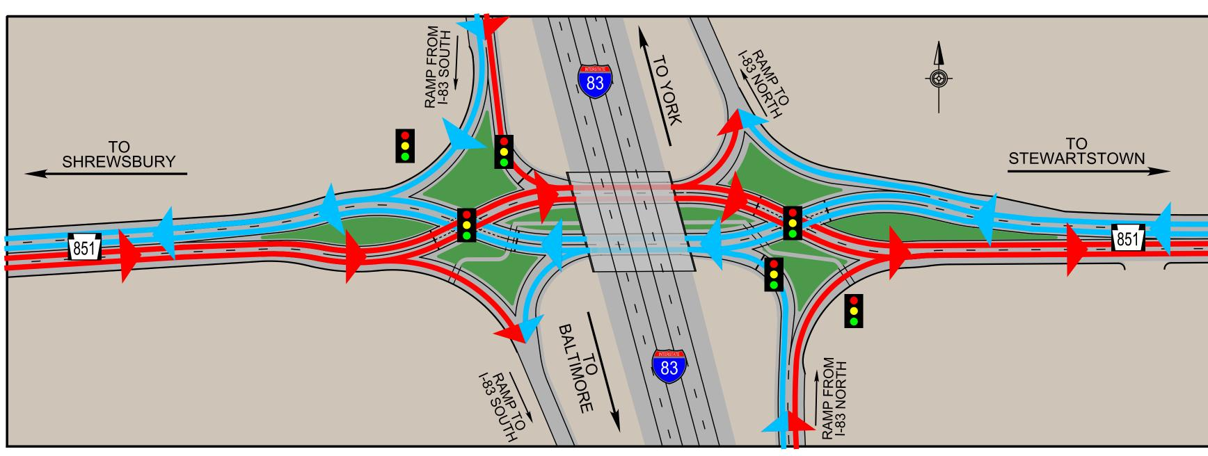
A diverging diamond interchange (DDI) is unique from a standard diamond interchange in that the side road traffic (PA 851), crosses over to the left side of the road at a signalized intersection prior to the bridge. This allows direct left turns from the off-ramps to merge and allows for a direct left turn on to the on-ramp. The side road (PA 851) traffic crosses back to the right side of the road at a signal beyond the bridge.
