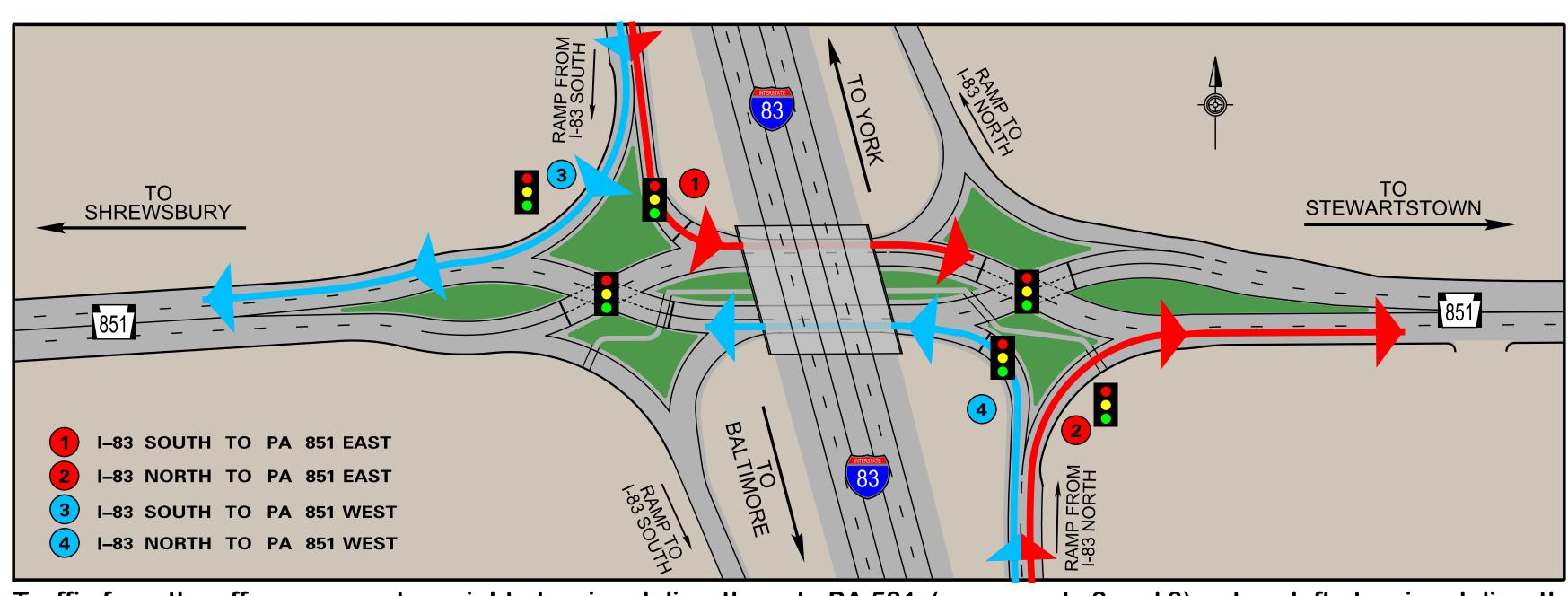
Traffic from the off-ramps can turn right at a signal directly on to PA 581 (movements 2 and 3) or turn left at a signal directly on to PA 581 (movements 1 & 4).
