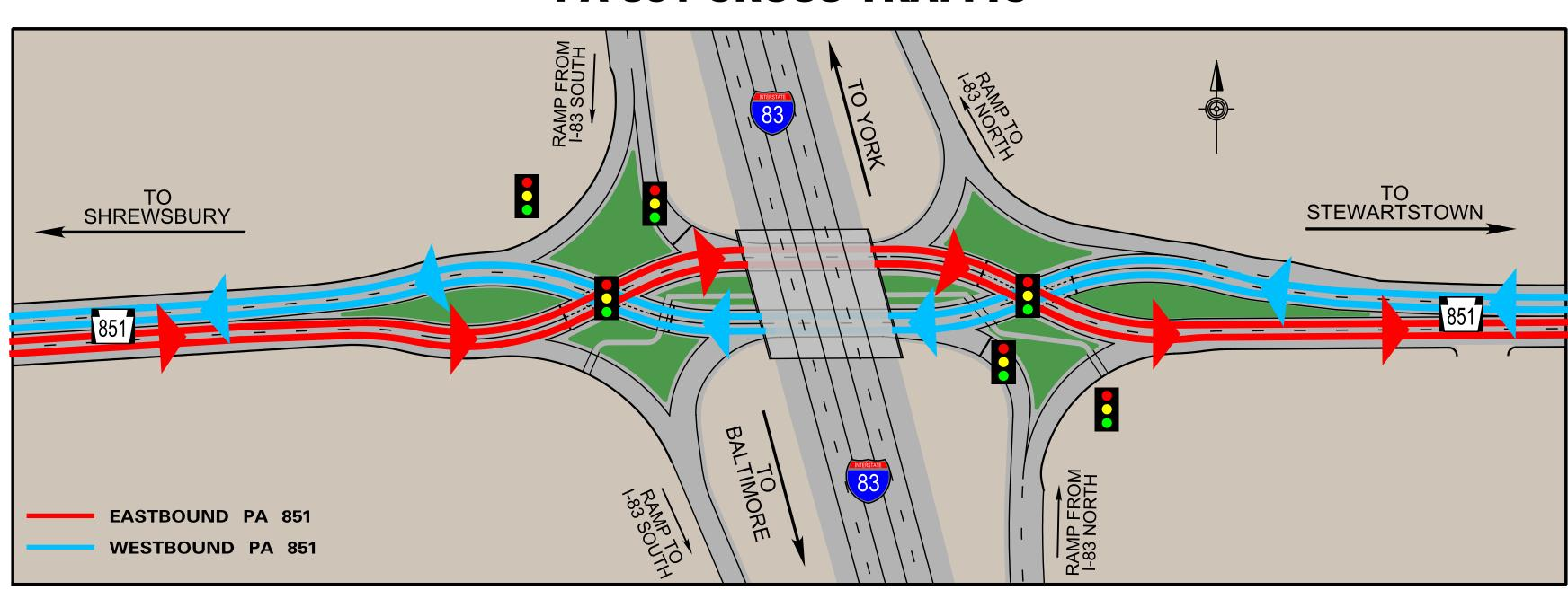
PA 851 traffic crosses over to the left side of the road at a signal prior to the bridge. It crosses back to the right side at a signal beyond the bridge.
