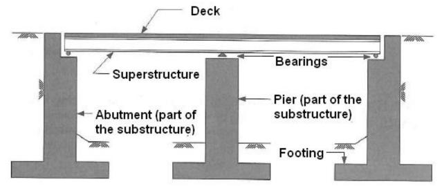
**Deck** = the part of a bridge that provides a surface for cars and pedestrians. **Superstructure** = the part of a bridge that supports traffic and transfers load to the bridge substructure below. Superstructure includes the beams or girders, railings, sidewalks, and bearings.
