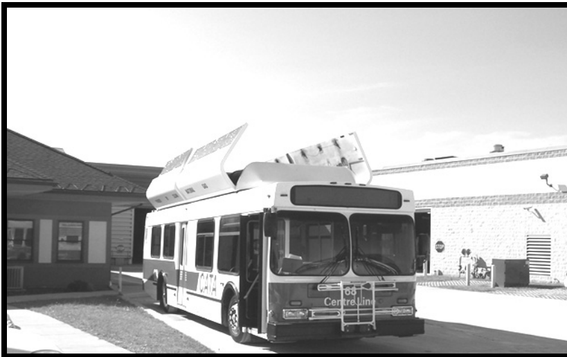
CATA Vehicle with Roof-Mounted Fuel Tanks
