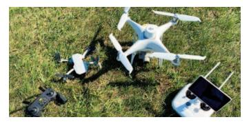
flight time using backup batteries. The operator uses the drone's camera to take high resolution photos and videos. Stabilizing systems in the drone keep the images clear and stable, even in a moderate wind. The drone's "home" function can be used to automatically return the drone to its takeoff location at any point during the flight to facilitate a safe landing.
